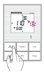
Press the : (Up) or : (Down) Key to adjust the cursor ' around the 24 hour clock in 30 minute increments. The 24 hour clock is displayed around the perimeter of the remote controller display screen.
