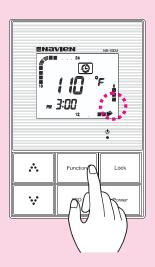
Move indicator '**II**' to a blacked block period and press the "FUNCTION" key to deactivate the recirculation pump for the current period. Repeat this action to clear multiple periods.
