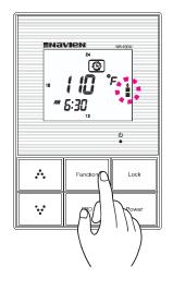
When you press the function button at a desired recirculation start time, a ' a' mark will appear meaning, that you are setting that time period for a circulation. After the black box mark appears, it will automatically go to the next time period, asking you if you want a circulation at that time, and so forth. You can manually press ".\*" or "\*.\*" to scroll to the time period that you want altered.
