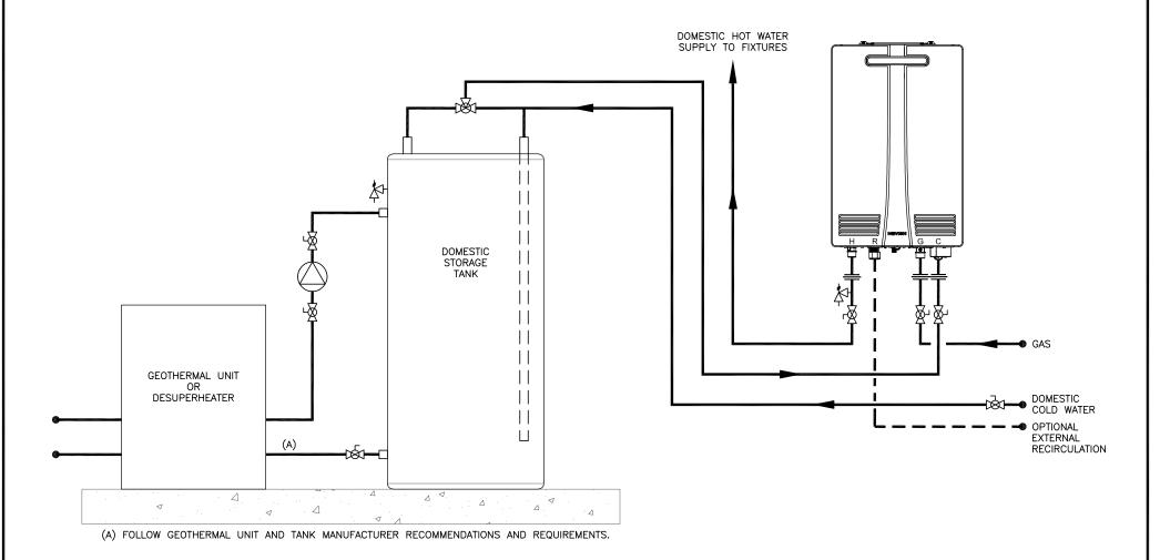
TANKLESS QUANTITY: RECOMMENDED PIPE SIZE 1 UNIT: 3/4" 2 UNITS: 1" 3 UNITS: 1-1/4" 4-5 UNITS: 1-1/2" 6-8 UNITS: 2" 9-14 UNITS: 2-1/2" 15-16 UNITS: 3" SYMBOL LEGEND
