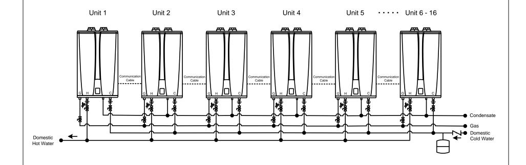
Recommended Pipe Size/Heater Count 1 Unit - ¾" 2 Units - 1" 3 Units - 1-¼" 4 to 5 Units - 1-½" 6 to 8 Units - 2" 9 to 14 Units - 2-½" 15 to 16 Units - 3"
