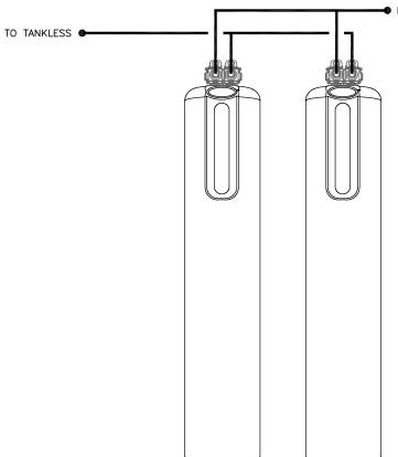
NUMBER OF PEAKFLOW C REQUIRED IS NOT EQUIVALENT TO NUMBER OF TANKLESS WATER HEATERS, PEAKFLOW C SIZING IS BASED ON FLOW RATE. SYSTEM DESIGN FLOW RATE IS 16 GPM PER TANK, 20 GPM PER TANK FOR INTERMITTENT USE ONLY. PEAKFLOW C CAN BE CASCADED UP TO 6 UNITS IN PARALLEL. PEAKFLOW IS NOT TO BE USED WITH TANK TYPE WATER HEATER OR TANK STORAGE. (REFER TO SIZING GUIDELINE FOR NAVIEN TANKLESS WATER HEATER ON NAVIENINC.COM)
