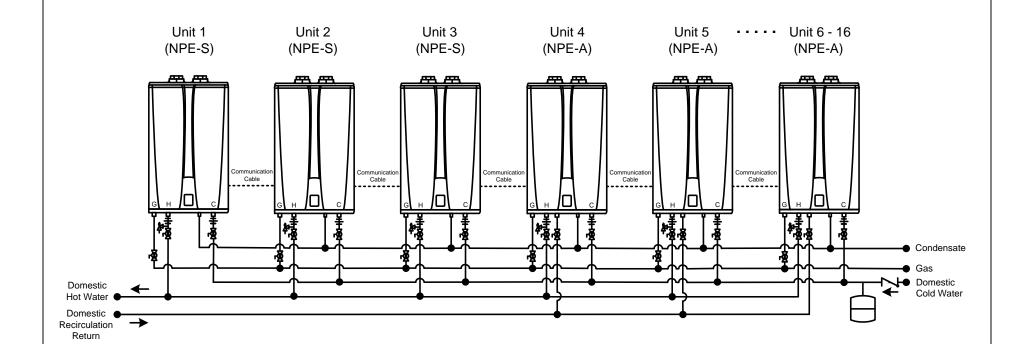
Recommended Pipe Size/Heater Count 1 Unit - 3/4" 2 Units - 1" 3 Units - 1-1/4" 4 to 5 Units - 1-1/2" 6 to 8 Units - 2" 9 to 14 Units - 2-1/2" 15 to 16 Units - 3"
