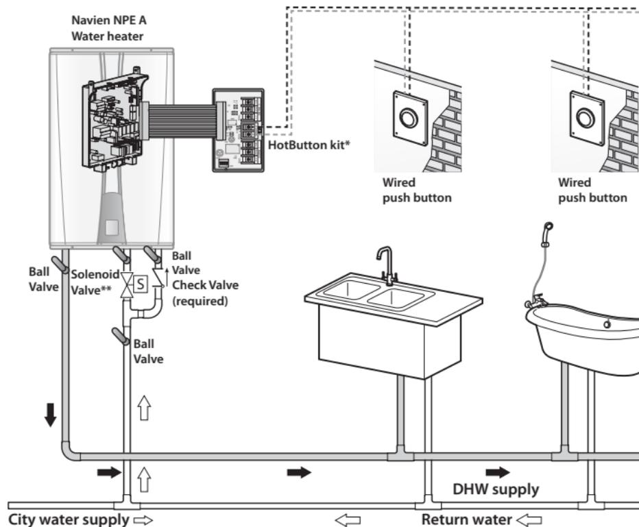
Install the recirculation valve to the faucet furthest from the water heater.
