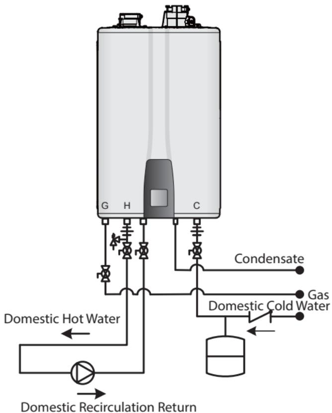
**[Type 2. Recirculation Using a Second Pump
