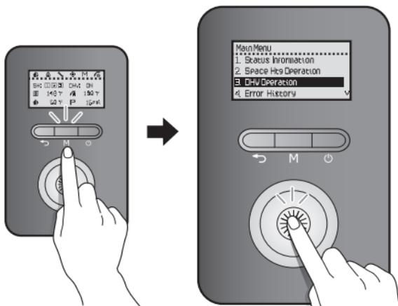
Rotate the Command dial (⊙) to switch between the list items or to increase/decrease setting values. Press the Command dial (⊙) to select an item or to confirm after making changes.
