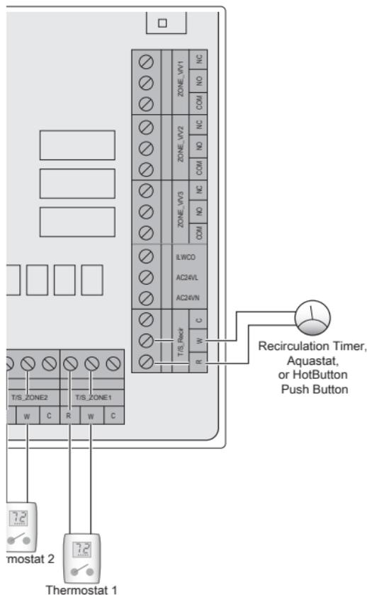
\* If the DHW recirculation menu is set to the Always On, Intelligent, or Weekly option, no aquastat or additional HotButton is required.
