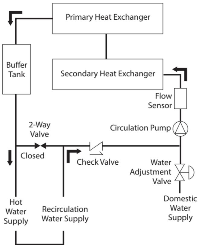
**[External Recirculation Mode using the Recirculation Inlet]**
