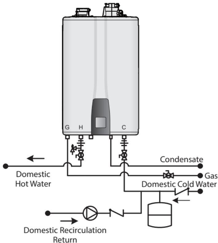
**[Type 1. Recirculation using External Pump -
