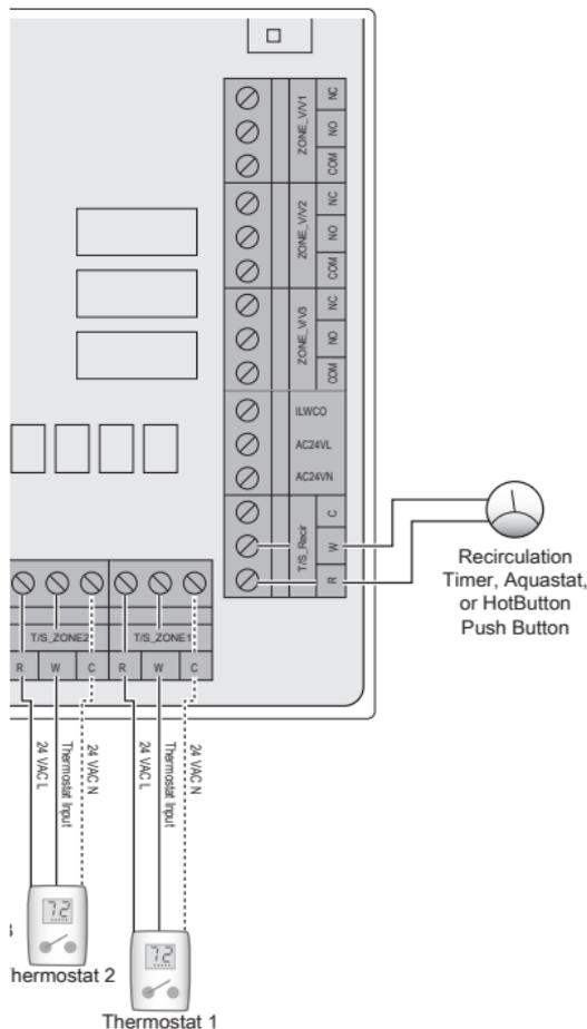
\* If the DHW recirculation menu is set to the Always On, Intelligent, or Weekly option, no aquastat or additional HotButton is required.
