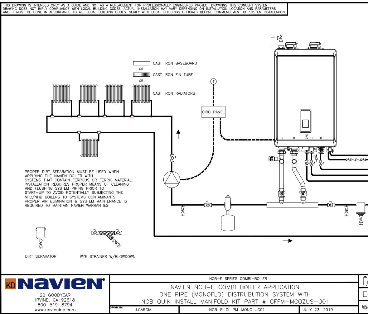
FIELD SUPPLIED CIRCULATOR ZONE PANEL SHALL HAVE DRY CONTACTS CLOSED ON HEAT CALLS WIRED TO NAVIEN NCB UNIT "T & T" TERMINALS TO ACTIVATE HEAT MODE DIP Sw 7 OF 8 Down (OFF) ON PCB
