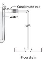
The end of the 1/2'' (NPT) plastic piping should drain into a laundry tub or into a floor drain.
