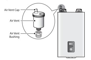
The Navien NFB boilers have a top connection for an air vent. An air vent must be installed to purge air from the boiler system.
