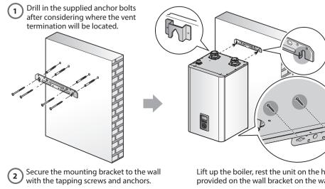
Lift up the boiler, rest the unit on the hooks provided on the wall bracket on the wall.
