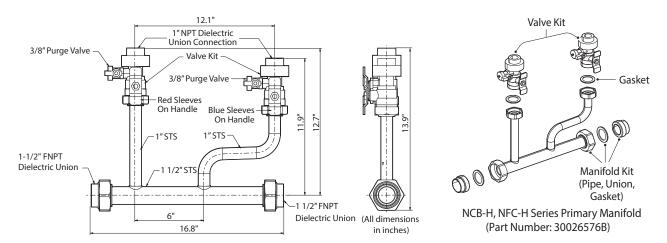
Check that a pipe, unions, gaskets, and valves are all included in the Manifold kit box and the Valve kit box. After installing the manifold and valve kits, ensure that the fittings, such as the unions and gaskets, are properly sealed with the pipe.
