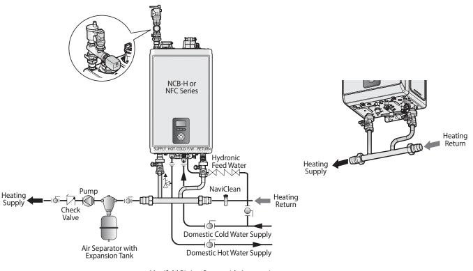
Manifold Piping Setup with Accessories
