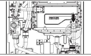
4. Remove the fastener clip labeled "22.3" (left) attached to the Heat Exchanger Outlet pipe, then loosen the clip to remove the Siphon Hose (right).
