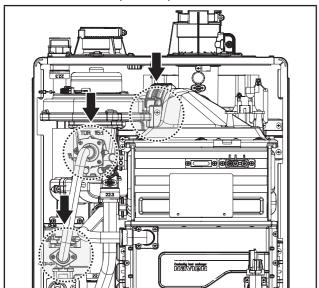
6. Remove the 4 screws attached to the brackets on either side of the Heat Exchanger Assembly.
