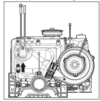
Insert new Fan Damper included with packaging in between where fan motor assembly and burner meet.
