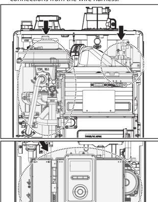
Remove fasteners labeled "22.3" and "19.2".
