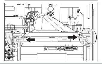
8. Remove the Ignition Transformer from the old assembly and install it onto the top bracket of the new replacement heat exchanger.
