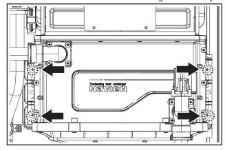
7. While supporting the weight from the bottom of the Heat Exchanger Assembly (approx. 30 lbs), remove the 5 screws attached to the top bracket.
