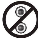
Do not vertically stack concentric terminations on sidewalls. The circulation of exhaust gases will cause improper operation of the boiler.
