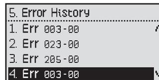
Rotate the Command dial (⌚) to switch between the list of errors. Press the Command dial (⌚) to select an error to view detailed information.
