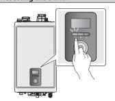
If an error message appears during boiler operation, reset the boiler to resolve the problem. Press the Back button () on the front panel to reset the boiler.
