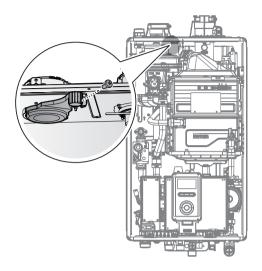
5. Pull the filter out of the boiler.
