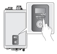
When the power is on, the boiler automatically enters normal operation mode, and the boiler's operating conditions are displayed on the screen.
