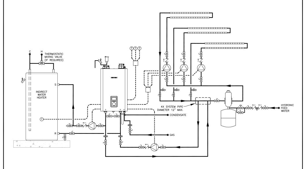
SYMBOL LEGEND EXPANSION TANK BACKFLOW PREVENTER FULL-PORT VALVE NFB-H SERIES BOILER MNavien THERMOSTA (1) NFB-H BOILER WITH MULTIPLE ZONE CIRCULATORS BALL DRAIN VALVE CONDENSATE TRAP AIR ELIMINATION AND INDIRECT WATER HEATER UNION 20 GOODYEAR IRVINE, CA 92618 INCLUDES MODELS NFB-175H, 200H COPPER BASEBOARD FIN TUBE 800-519-8794 Ŵ S. STOEKE NFB-H-1-3ZP-IDWH MAY 24, 2022 www.navieninc.com
