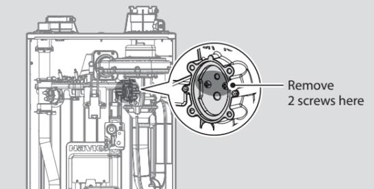
Figure 4. Access to Gas Orifice in Fan Assembly
