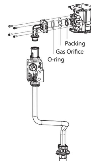
Figure 5. Exploded View of Gas Pipe Assembly
