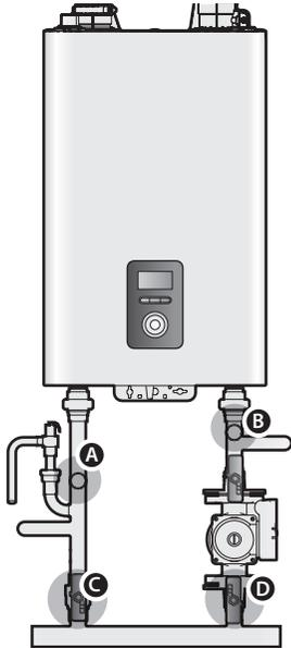
To flush the Heat Exchanger:
