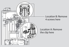
Figure 3. Detaching the Gas Valve Outlet Adapter from the Gas Valve and Fan Motor Assembly
