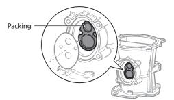
9. Replace the gas valve outlet adapter to its original position and use all screws to secure all connections.
