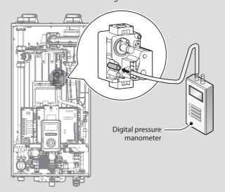
Figure 8. Connect Digital Pressure Monometer
