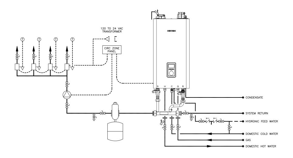
SYMBOL LEGEND BACKFLOW PREVENTER FULL-PORT VALVE NFC-H SERIES COMBI-BOILER MNavien THERMOSTA (1) NFC-H COMBI-BOILER WITH MULTIPLE ZONE VALVES AIR ELIMINATION SHOWN WITH NAVIEN MANIFOLD KIT PART#30026576B ZONE VALVE MANIFOLD 20 GOODYEAR IRVINE, CA 92618 INCLUDES MODELS NFC-250/175H, NFC-250/200H 800-519-8794 BALL DRAIN VALVE S. STOEKE NFC-H-1-ZP-4ZV-PLSS MARCH 7, 2023 www.navieninc.com
