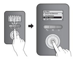
A list of 10 recent errors are displayed on the screen, with the most recent error displayed at the top of the list.
