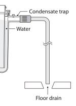
The end of the 1/2'' (NPT) plastic piping should drain into a laundry tub or into a floor drain. æ
