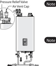
Prior to connecting piping to the boiler, flush Note the entire system to ensure it is free of sediment, flux, scale, debris or other impurities that may be harmful to the system and boiler. During the assembly of the
