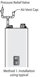
The following figure illustrates an example of installation using the PRV-air vent adapter.
