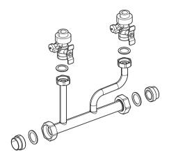
Also, check that a pipe, unions, gaskets, and valves are all included in the Manifold kit. After installing the manifold, ensure that the fittings, such as the unions and gaskets, are properly sealed with the pipe.
