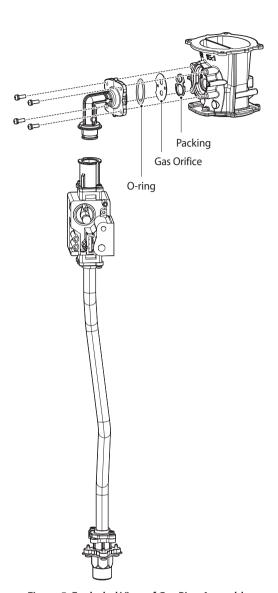
Figure 5. Exploded View of Gas Pipe Assembly
