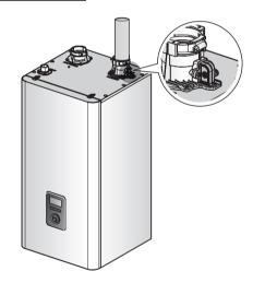
As shown, the VID is a device connected to the vent collar which is intended to detect whether the vent pipe has been inserted to a sufficient depth into the collar during its initial installation.
