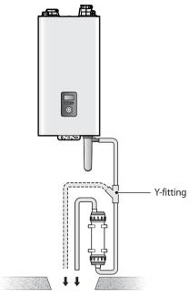
Figure 2. Vertical installation
