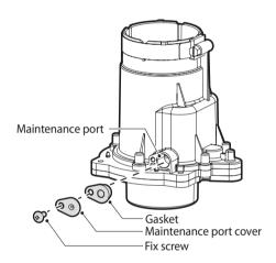
Refer to "9.8 Maintenance" for detailed inspection procedures of the Navien Common Vent Collar Kit (Back-draft Damper).
