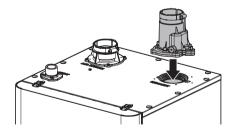
4. Tighten the four mounting screws to secure the Common Vent Collar Kit in place. The screws (x 4) are supplied with the Common Vent Collar Kit.
