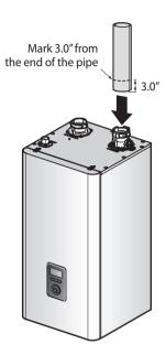
2. Insert the pipe into the vent collar to start the vent run. Make sure to completely slide the vent into the collar until the end makes contact with the bottom of the socket.
