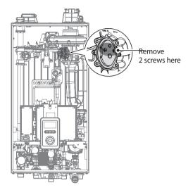
Figure 4. Access to Gas Orifice in Fan Assembly
