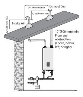
• Non-Concentric Sidewall Venting - Air is drawn from a different location that is at least 12 in (300 mm) away from the exhaust termination. The exhaust termination can be located either on the sidewall or roof. Try to minimize the length of the intake air pipe when installing the vent.
