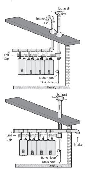
To install a condensate drain to the common vent system:
