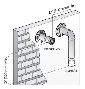
In cases where a 12" horizontal clearance is not possible, provide a vertical clearance of at least 36" with the exhaust above the intake but do not exceed 20'.
