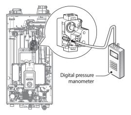
Figure 9. Connect Digital Pressure Monometer
