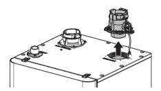
3. Connect the Common Vent Collar Kit to the exhaust duct of the boiler unit.
