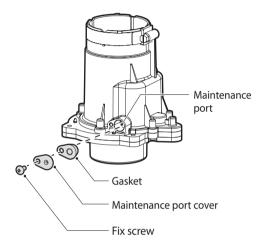
2. Through the maintenance port, check the operating condition of the damper plate inside the Common Vent Collar Kit.
