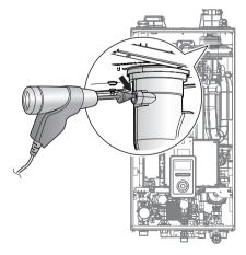
Figure 7. Insert the Analyzer
