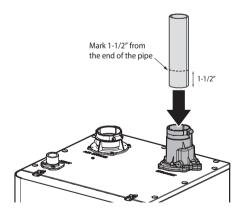
Insert the vent pipe into the vent collar to start the vent run. Make sure to completely slide the vent into the collar until the end makes contact with the bottom of the socket.
