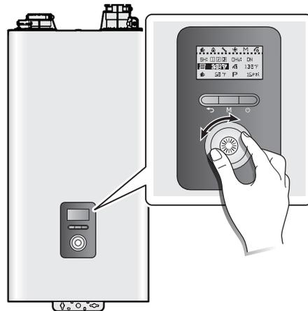
2. Press the Command dial (⌚) to select the space heating temperature. The highlighted section will flash.
