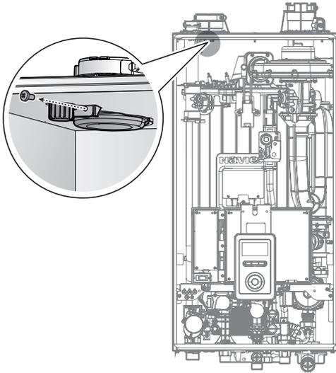
6. Remove the filter from the plastic assembly. Dust and rinse it with clean running water.
