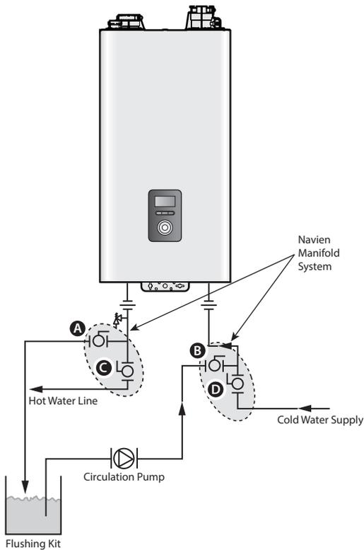
10. Rinse the cleaning solution from the boiler:
