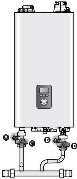
1. Press the Power button (⏻) on the front panel to turn off the boiler.
