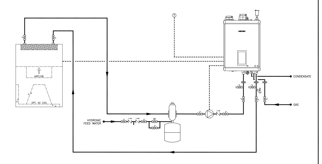
SYMBOL LEGEND BACKFLOW PREVENTER FULL-PORT VALVE NHB-H SERIES BOILER MNavien THERMOSTAT ---- CONTROL WIRING (1) NHB-H BOILER WITH AIR HANDLER PRESSURE REDUCING VALVE BALL DRAIN VALVE Ŵ AIR ELIMINATION = 20 GOODYEAR INCLUDÉS MODELS NHB-55H, 80H, 110H, 150H IRVINE, CA 92618 800-519-8794 AUTOMATIC AIR VENT S. STOEKE NHB-H-1-AH JANUARY 11, 2024 www.navieninc.com
