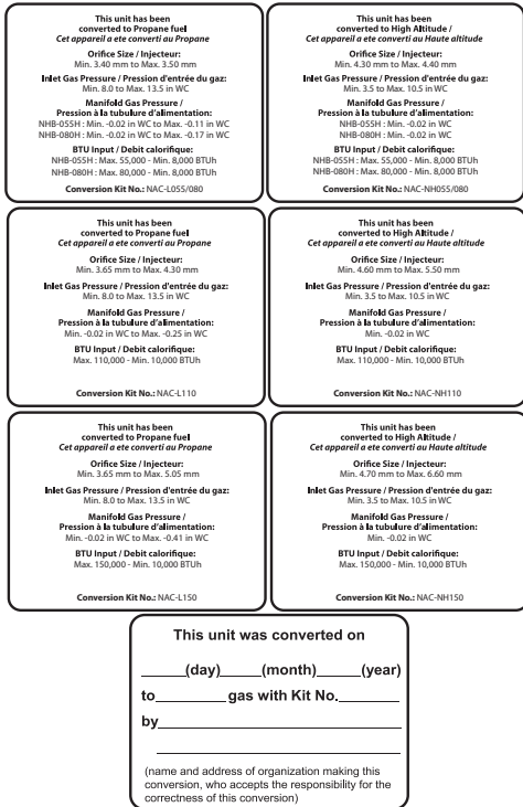
Figure 11. Proper Placement of Gas Conversion Labels
