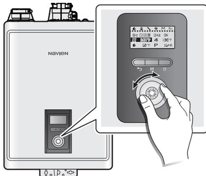
2. Press the Command dial (☀️) to select the desired zone, and then press the Command dial (☀️). The selected zone's temperature will flash.
