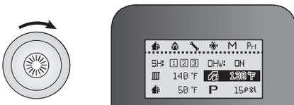
3. Press the Command dial (🌀) to select the indirect DHW temperature (🌀). The highlighted section will flash.
