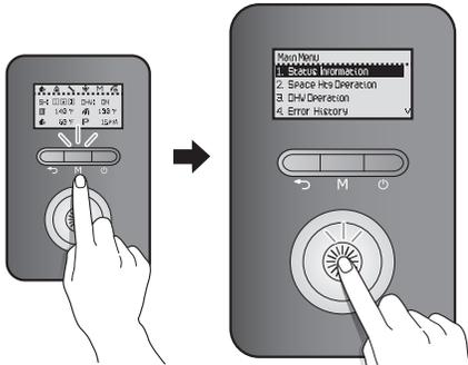
Rotate the Command dial (⊙) to switch between the information items. Press the Command dial (⊙) to select an item and view the information.
