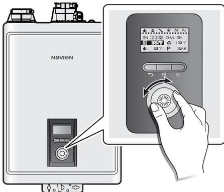
2. Rotate the Command dial (🌀) to the right to select the DHW temperature.
