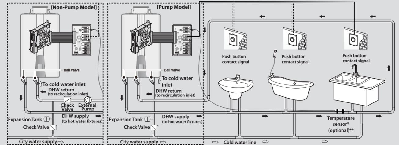
\* When the temperature sensor is installed, it must be insulated. The sensor wire may be extended by up to 100 ft (30 m) using 22AWG wire.
