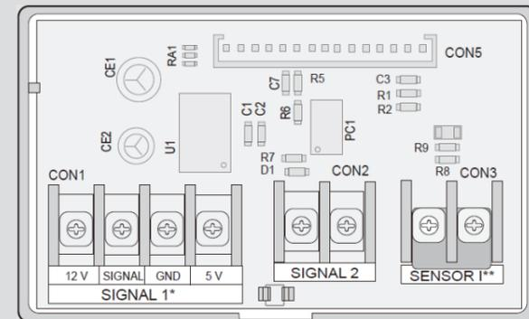
\* SIGNAL1 contacts are for optional wireless push buttons or motion sensor accessories.
