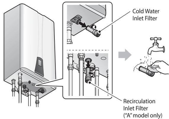
3. Reinsert and tighten the filters.
