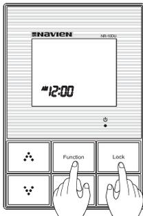
Get into setting mode by pressing the “Function + Lock” buttons simultaneously for 3 seconds in power off status.
