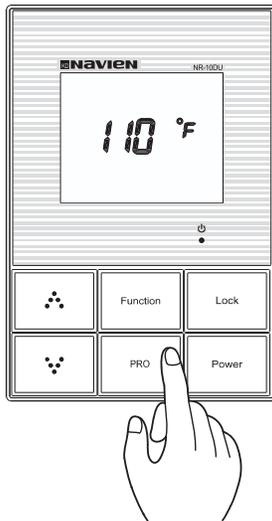
When the Pro Key is pressed for 5 seconds, high temperature adjustment mode is readied.
