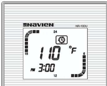
For example, recirculation could be set to run from 6AM to 9AM and from 6PM to 9PM daily- see screen sample on the left side.
