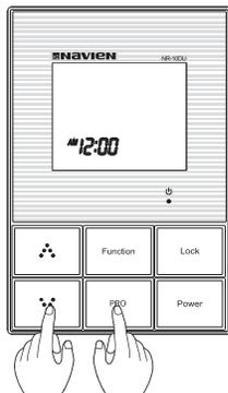
A Remote Controller can be put back to power off mode by pressing the “⏮(Down) + PRO” buttons simultaneously for 3 seconds.
