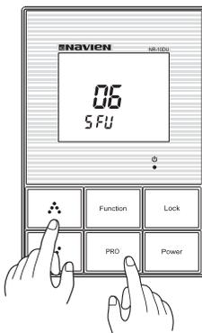
When you press the “
