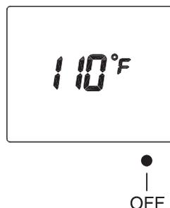
When the hot water faucet is closed, the water heater turns off automatically. The GREEN LED indicator turns off.
