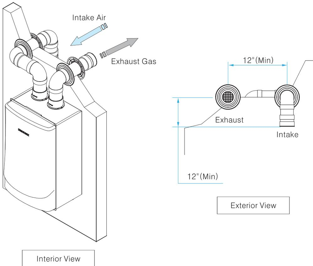
**Option #2: Non-concentric venting through a side wall. Air is drawn from different location at a minimum of 12" from the termination. Please try to minimize the length of the intake air pipe length.**
