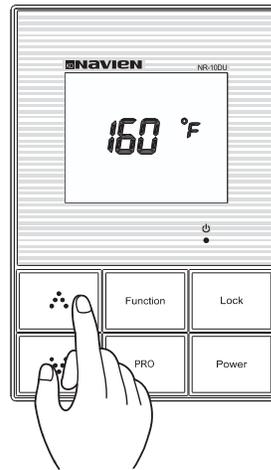
Each time Pro Key is pressed for 5 seconds in high temperature adjustment mode, temperature increases by 10°F (140~180°F) or 5°F (180~185°F). When the desired temperature is reached, leave alone and it will automatically set.
