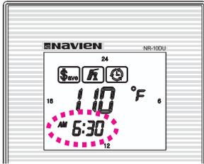
Before setting the Recirculation timer, ensure the remote controller is set to the current time. If the clock is not set to the current time, please adjust the clock (refer to 74 page).
