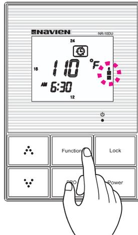
When you press the function button at a desired recirculation start time, a '■' mark will appear meaning, that you are setting that time period for a circulation. After the black box mark appears, it will automatically go to the next time period, asking you if you want a circulation at that time, and so forth. You can manually press "⬆" or "⬇" to scroll to the time period that you want altered.
