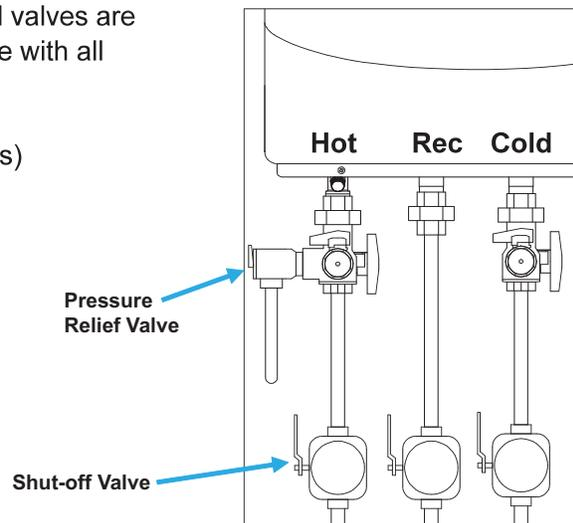
Instructions for pressure, temperature and vacuum relief valves shall specify that no valve is to be placed between the relief valve and the tank. The instructions shall specify installation in such a manner that the discharge from temperature and pressure relief valves will be conducted to a suitable place for disposal when relief occurs and that no reducing coupling or other restriction be installed in the discharge line.
