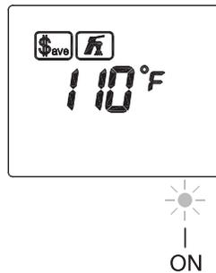
When a hot water faucet is opened, the unit will automatically start. The GREEN LED indicator will illuminate indicating normal operation.
