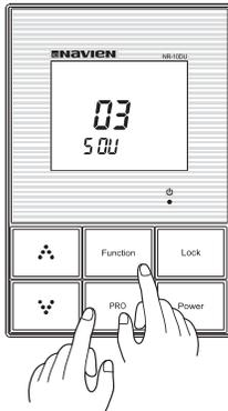
With the power off, when you press the “Function”, and “Pro” keys together for 3 seconds, you will see a “S OU” on the screen and the cascade On unit setup value when using the cascade function near the temperature is indicated.
