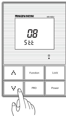
Press the “▲” or “▼” button to adjust the storage tank temperature. The value will be within the cascade OFF unit range and adjustable by 1.
