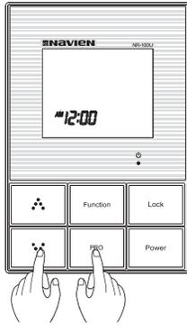
Get into setting mode by pressing “⏮(Down) + PRO” buttons simultaneously for 3 seconds in power off status.
