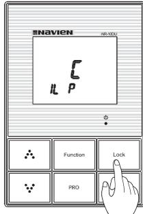
When in setting mode, “IL P” is displayed on the lower left side of the screen. If a Remote Controller is in setting mode “S” is displayed on the lower left side of the screen. If a Remote Controller is not in setting mode, “C” is displayed on the lower left side of the screen.
