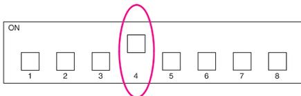
Dip-switch setting for Internal Recirculation mode
