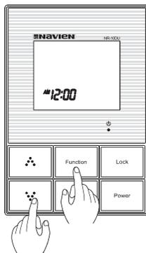
A remote controller can be put back to power off mode by pressing the “Function + Down” buttons simultaneously for 3 seconds.
