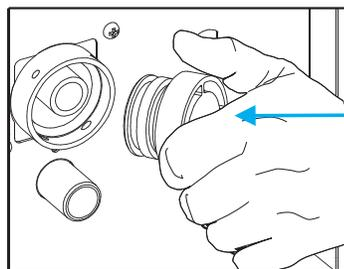
Prepare bucket; twist and remove cap; drain, clean out siphon and re-insert cap and retaining clip.
