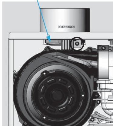
3. Remove the filter from the bottom of the intake air duct. Remove the Intake air filter from the plastic assembly and clean it with a toothbrush and water. Re-fit the screen into the plastic assembly and fit the filter and frame onto the bottom of the intake air duct.
