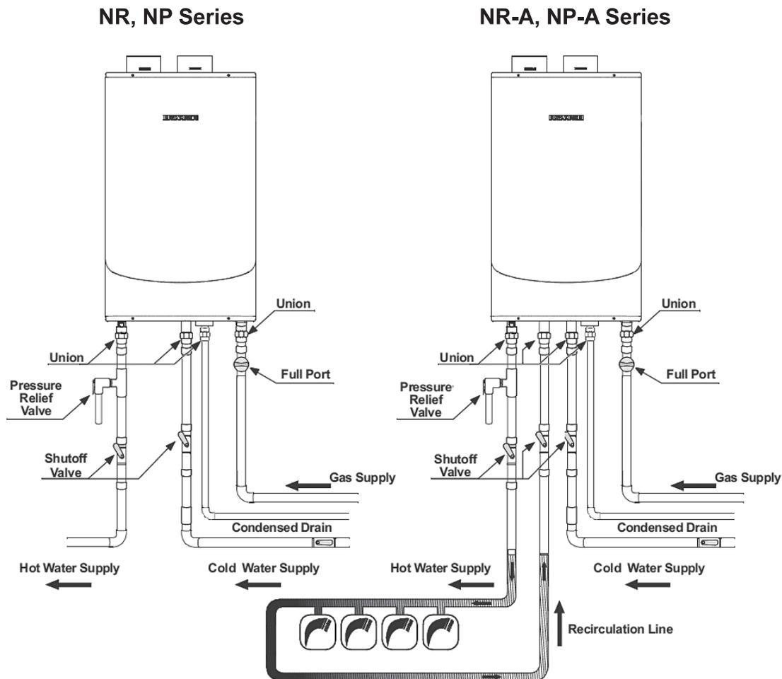
**NOTICE :** If using mixing valves on the outlet, choose one which prevents cold water pressure from overcoming hot water line pressure.
