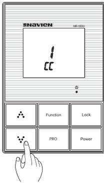
“CC” is displayed near where the ‘minute’ side of the clock on the LCD screen (lower left side) in setting mode. And the current number of initial activating water heaters is displayed near where temperature is displayed (center of screen).
