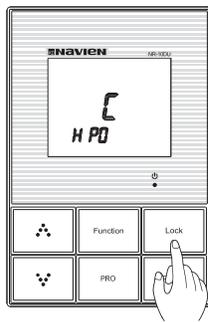
When in setting mode, “HPO” is displayed near where ‘minute’ of clock is usually displayed (lower left side). If a Remote Controller is in setting mode “S” is displayed near where the temperature is usually displayed (center of screen). If a remote controller is not in setting mode, “C” is displayed near where temperature is usually displayed (center of screen).
