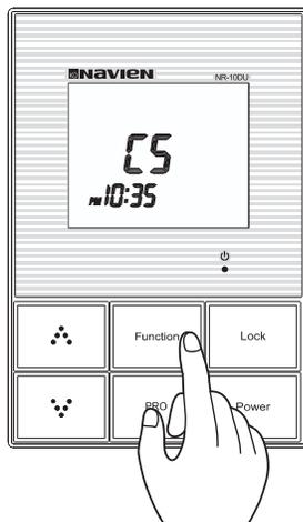
Once the “Function” button is pressed, “AM/PM” flashes on the display. Use the ▲(Up) or ▼(Down) buttons to select AM or PM. After 3 seconds, the selection is automatically set.
