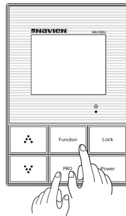
When you press the “Function” button and “Pro” button for 3 seconds, the setup mode will be over and it enter the power off mode.
