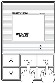
A remote controller can be put back to power off mode by pressing the “Function + Lock” buttons simultaneously for 3 seconds.
