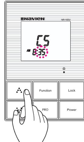
Use the ▲(Up) or ▼(Down) buttons to scroll until the desired minute time is reached. Press the “Function” button to set.
