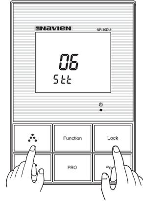
\*S tt : Setting temp-gap of storage tank
