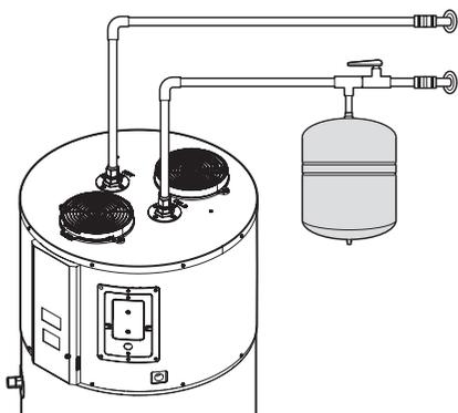
**Note** There may be a check valve, pressure-reducing valve, water meter, or water softener in the cold water supply line, which can create a closed-loop system. Check if a check valve is installed in the cold water supply line of the water heater. If so, install an expansion tank between the check valve and the water heater.
