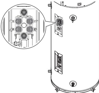
5. Separate the ECO switch from the ECO bracket to remove it.
