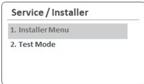
2. In the Password screen, press the Up button (▲) or the Down button (▼) to change numbers and places and press the OK button (OK) to enter the password. If the password is correct, the Installer Menu will be displayed.
