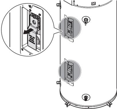
4. Remove the 4 screws on the ECO wires, 2 bolts on the ECO bracket from the water heater. Then, disconnect the wires from the ECO switch.
