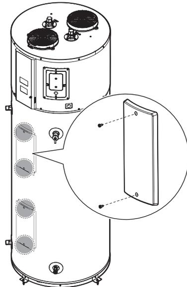
3. Remove the safety cover by pulling it forward.
