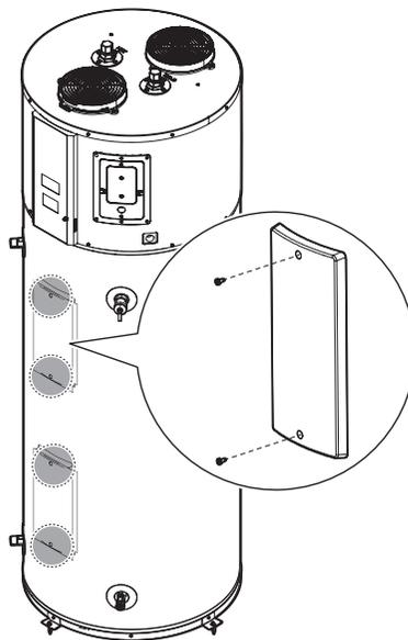
4. Remove the safety cover by pulling it forward.
