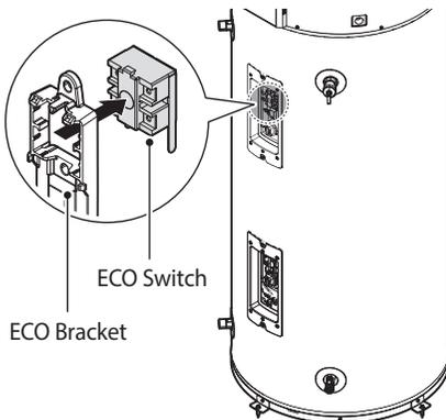
6. Replace with a new ECO switch, connect the 4 ECO wires to the ECO switch using 4 screws, then install both the safety cover and heating element cover on the water heater.
