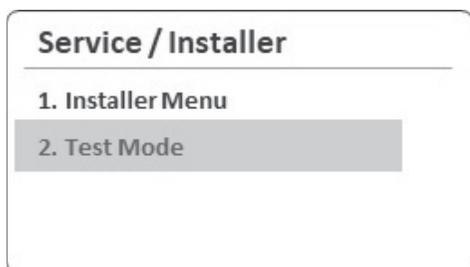
2. Press the Up button (▲) or the Down button (▼) to switch between the items. Press the OK button (OK) to verify the proper operation for the system component.
