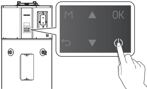
When the power is turned on, the product performs the Self Diagnostic operation. (This operation is performed each time the power is turned on after being in an unpowered state.)
