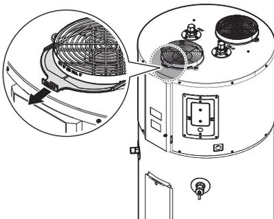
3. Remove dust or debris from the filter using water or a vacuum cleaner.
