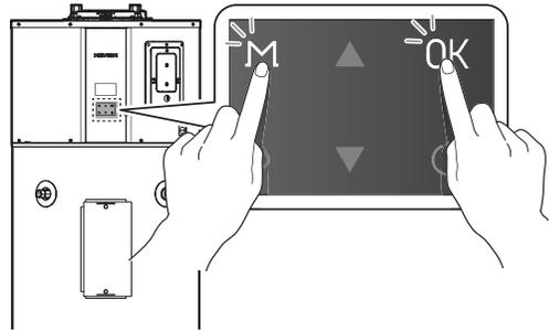
6. When the guidance screen appears, press the OK button (OK).
