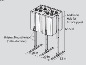
The water heater or boiler units can be mounted using the inline or back-to-back setup.
