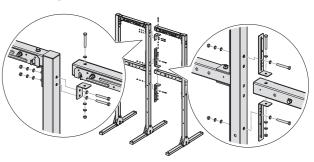
Refer to the instructions on pages 5 to 8 to connect an additional extension rack to the single frame with the fixed brackets and M10 bolts (3 in).
