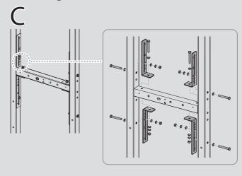
Place a fixed bar between the middle of the two post bars and four fixed brackets (middle) with six M10 bolts (3 in) to attach the middle bar.
