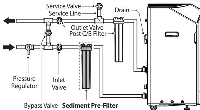
Refer to the following for changing the cartridge in the sediment pre-filter.
