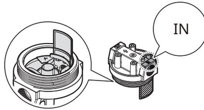
11. Make sure the cartridge is centered in the filter housing and tighten using the filter housing wrench.
