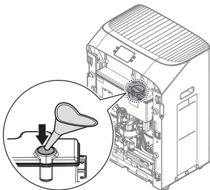
4. Fill the CIP tank with CIP solution using the funnel.
