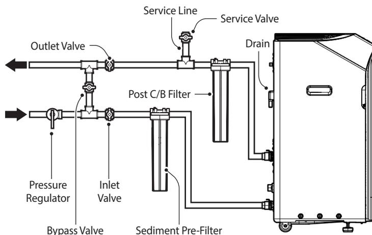
2. Half-open the outlet valve and cold-water faucet closest to the WEC.
