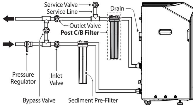
Refer to the following for changing the cartridge in the post carbon block (C/B) filter.
