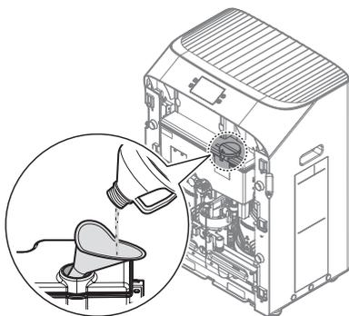
**Note** After using the funnel, wash it with water to remove any remaining CIP solution.
