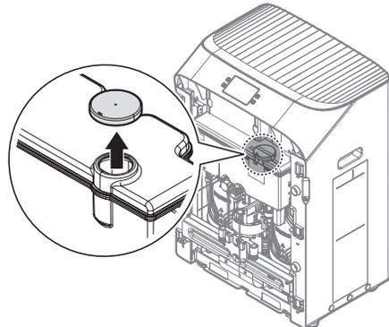
3. Insert a funnel into the CIP tank inlet.
