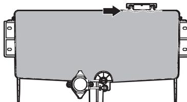
6. Close the front cover and tighten both screws.
