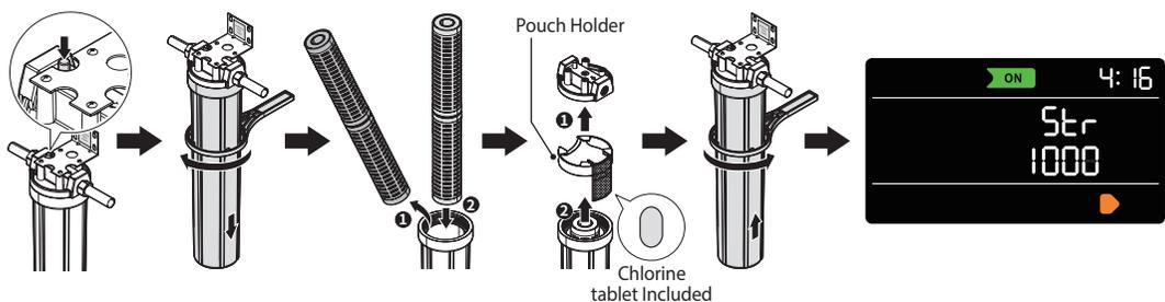
1. Press and hold the [Back] and [Next] buttons simultaneously for 3 seconds to enter Installer Setting mode and enter STR mode to clean the inside of the product. For more details, refer to “3.8 Using Installer Setting Mode” on page 33.
